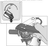
Make sure the float moves freely after this adjustment has been carried out, or the inlet valve will not shut off or will be in shut off position.
