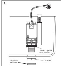
Position the Valve inside the tank ensuring the 10mm internal seal washer is on the thread shank first.
