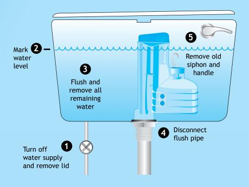
**Note:** Ensure the top of the new variflush valve is below the lowest overflow point of the cistern including all apertures.
